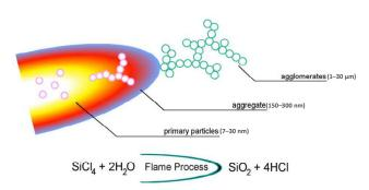
$SiCl_4$  in gas phase reacts spontaneously and quantitatively in an oxy-hydrogen flame with the intermediately formed water to produce  $SiO_2$  molecules.
